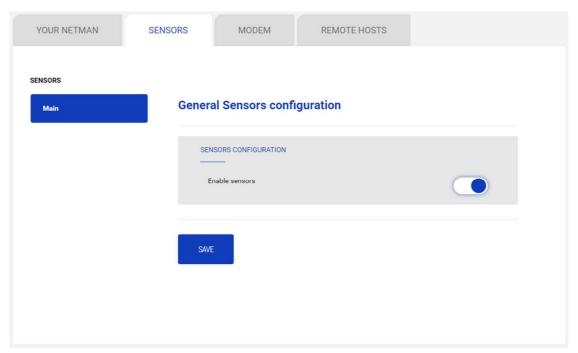
Enable the sensors and press on SAVE. Then, to detect all of the sensors connected to the Netman 208, select START SCAN.
